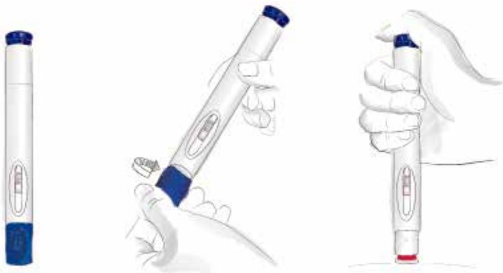
Fig 2. Designing devices with human factors considerations: The cap for this device was designed with a fingerprint-like extrusion to help patients with dexterity issues to enhance their grip. The cap also offers different ways of uncapping (twisting or pulling) giving the user increased flexibility with cap removal
